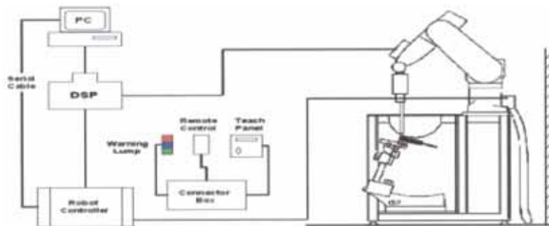
Figure2. SAR Lab Test Measurement Set-up
