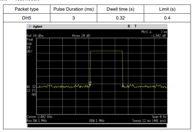
Note: for the worst mode of DH5 packet type, in normal hopping mode, hopping rate is 1600hops/s with 6 slots in 79 hopping channel
