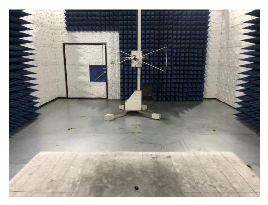
RADIATED EMISSION TEST SETUP ABOVE 1GHZ
