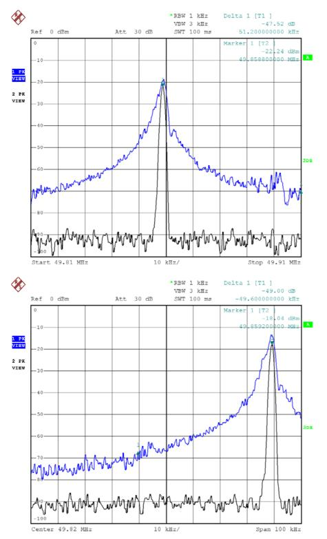
Bandwidth /-Bandedge Plot - Pursuant to FCC Part 15 Section 15. 235 Requirement (Pass/Fail)
