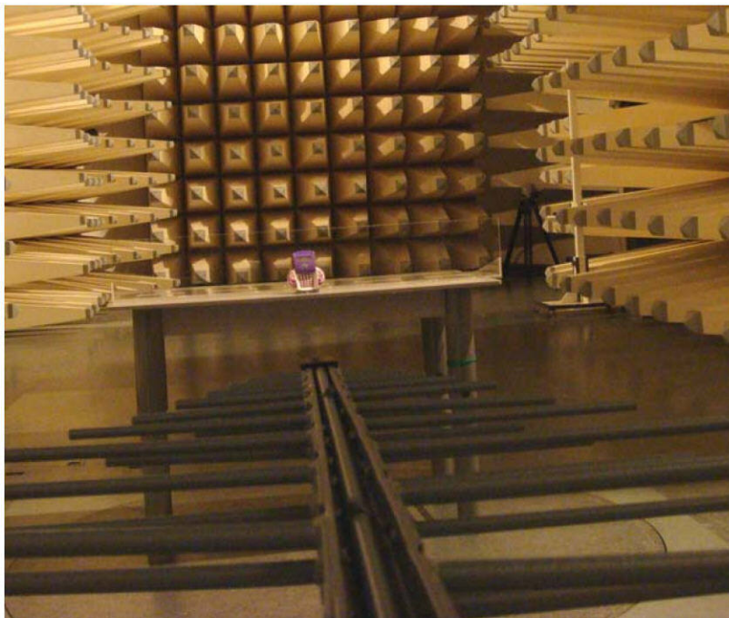
3m Measurement distance in semi anechoic chamber
