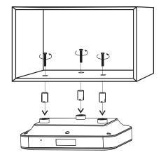
Use and follow the instructions on the included Mounting Template when attaching to the underside of your cabinet.
