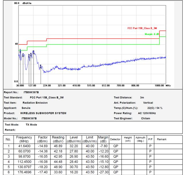
Note: Below 30MHz, the emissions are lower than 20dB below the allowable limit.
