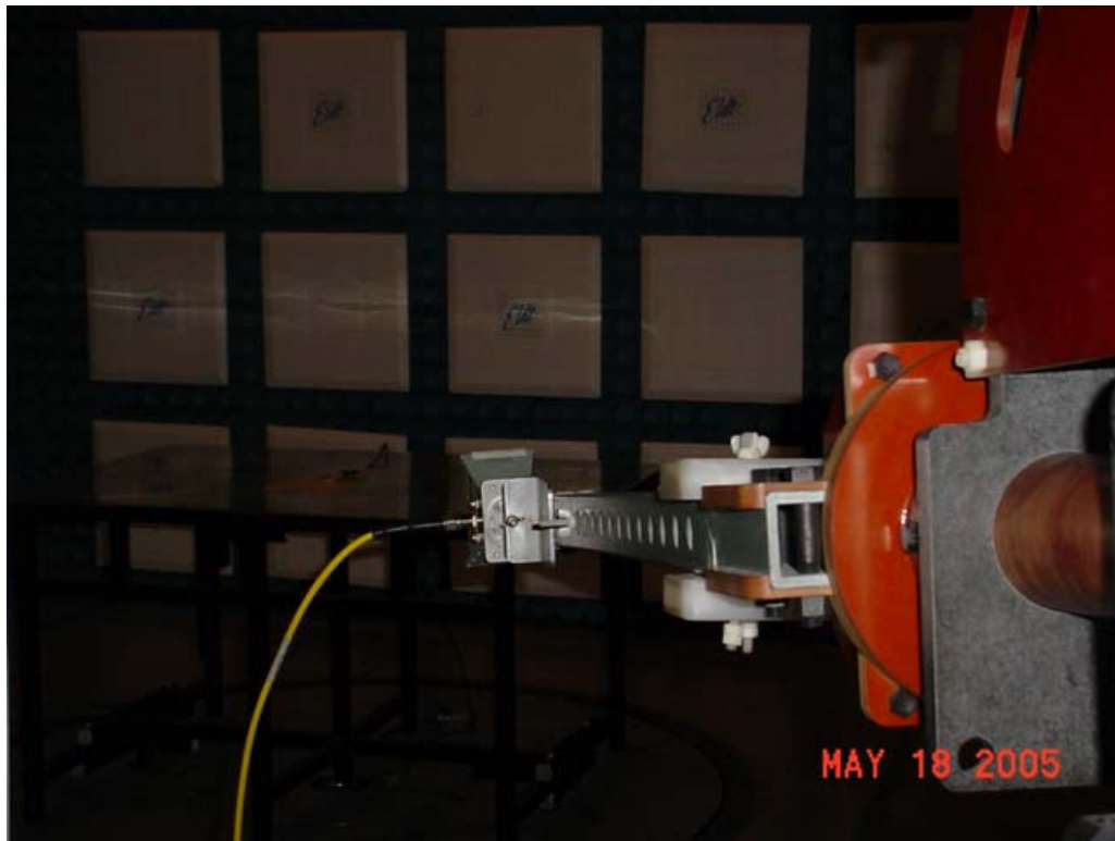
Test Setup for Radiated Emissions – Horizontal Polarization
