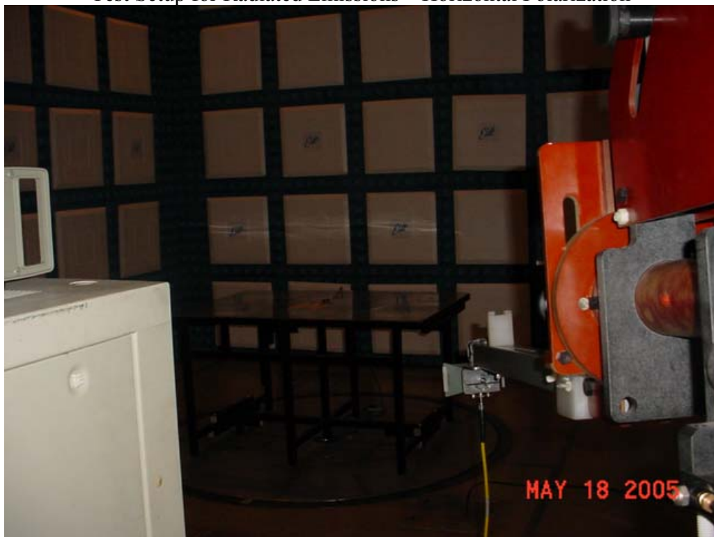
Test Setup for Radiated Emissions – Vertical Polarization
