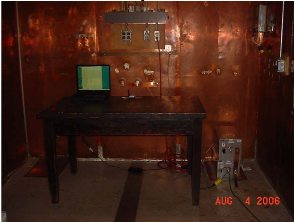
Test Set-up for Conducted Emissions
