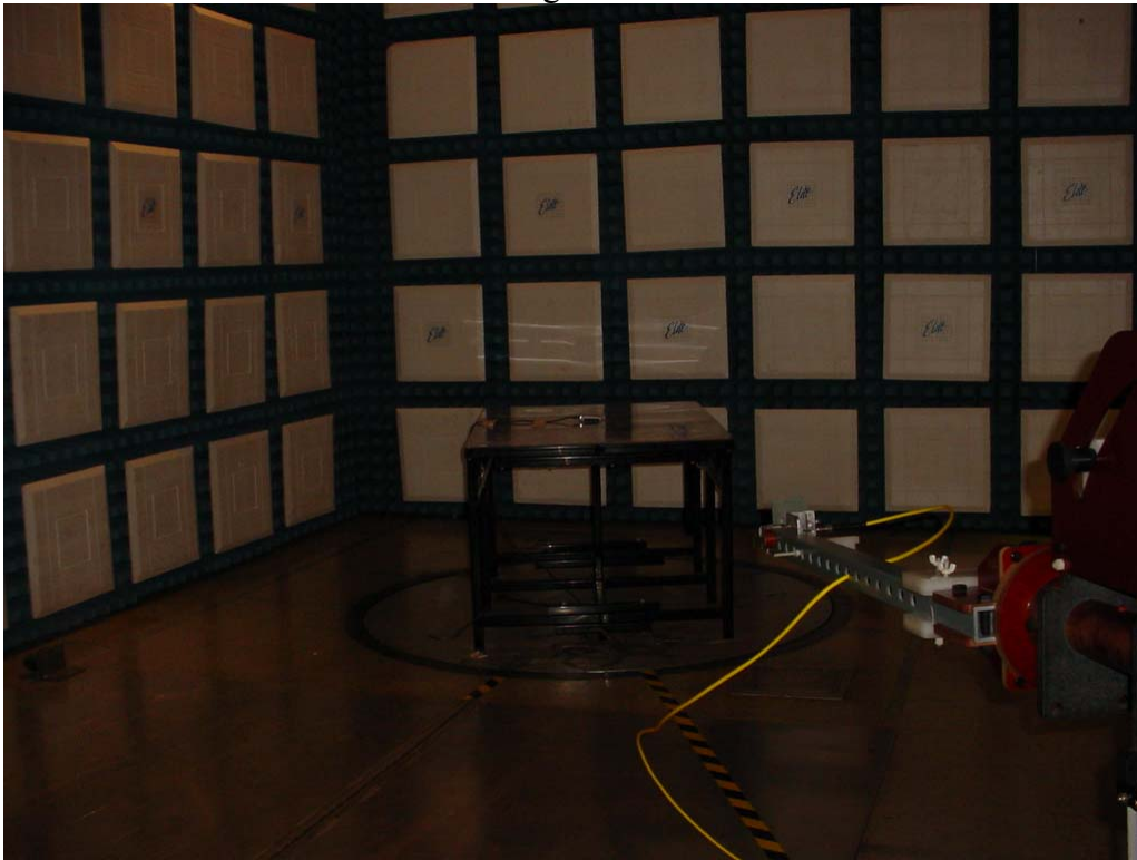
Test Set-up for Radiated Emissions – Horizontal Polarization
