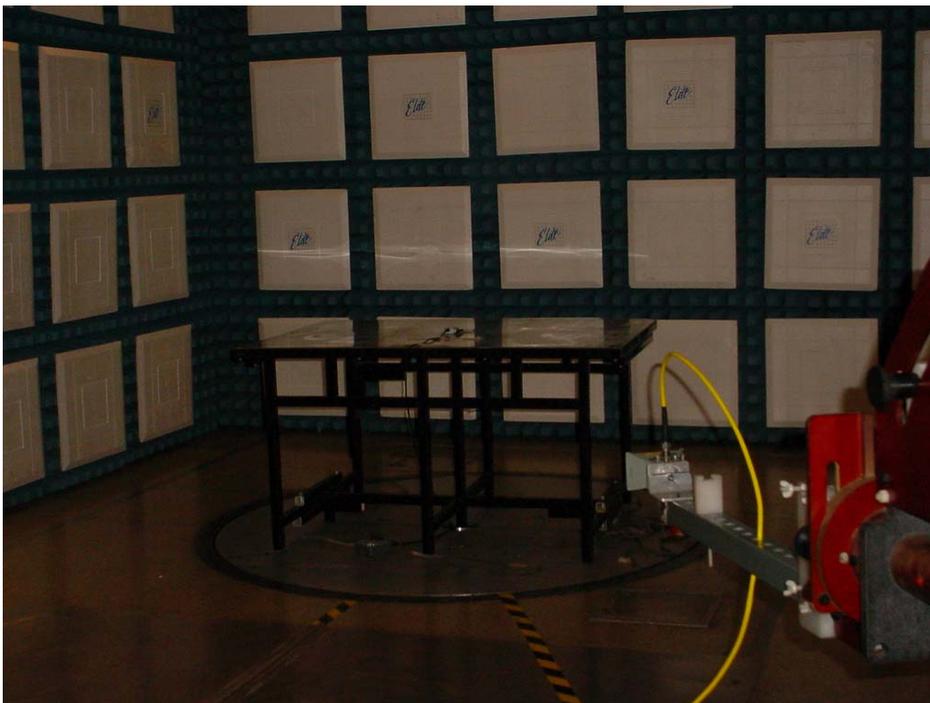
Test Set-up for Radiated Emissions – Vertical Polarization
