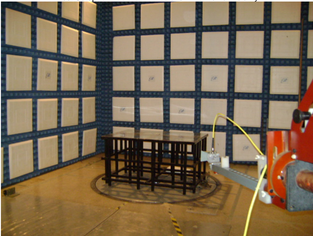
Test Setup for Radiated Emissions – Vertical Polarity
