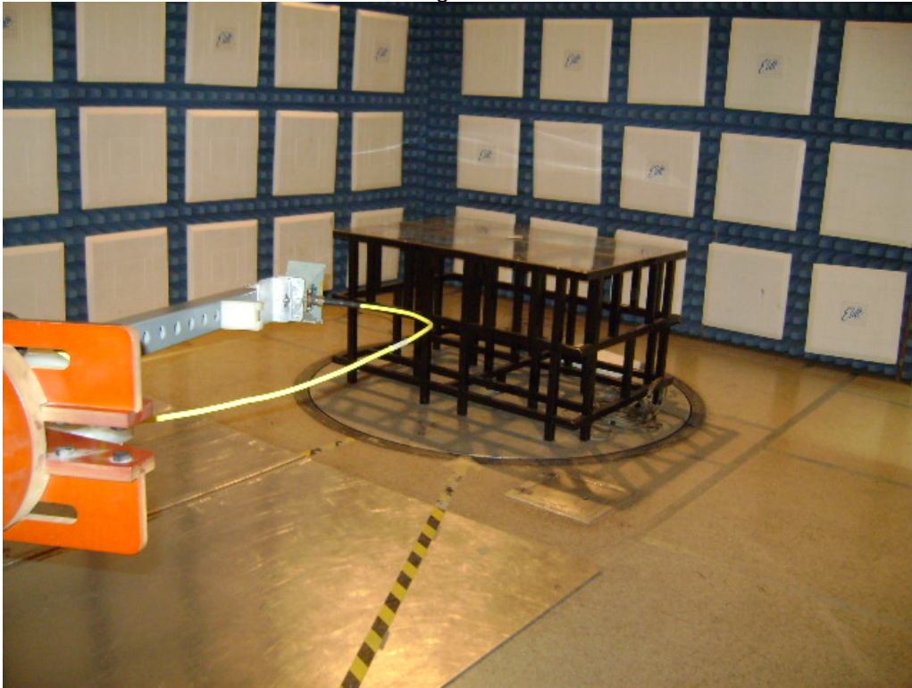
Test Setup for Radiated Emissions – Horizontal Polarity
