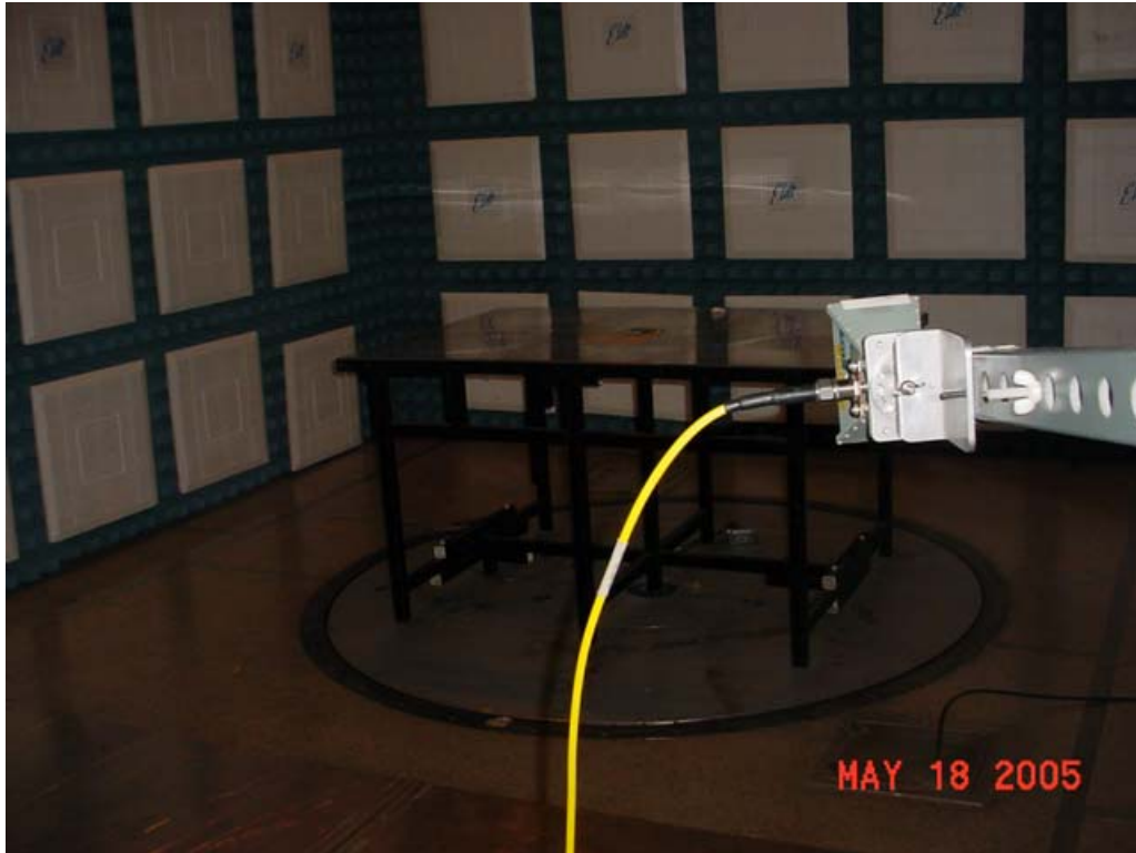
Test Setup for Radiated Emissions – Horizontal Polarization
