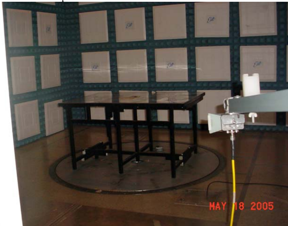
Test Setup for Radiated Emissions – Vertical Polarization
