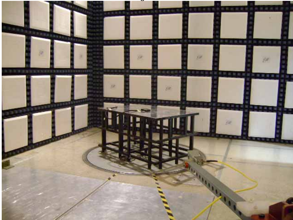
Test Setup for Radiated Emissions – Horizontal Polarity
