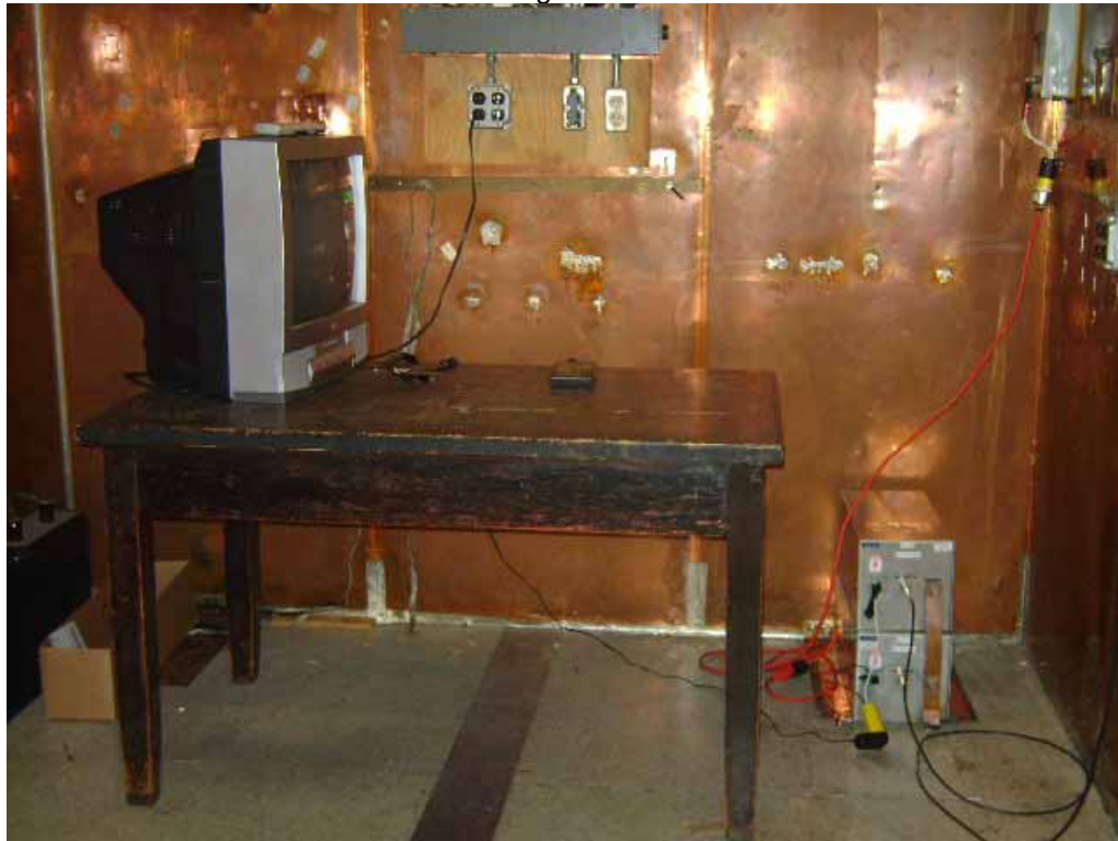
Test Setup for Conducted Emissions
