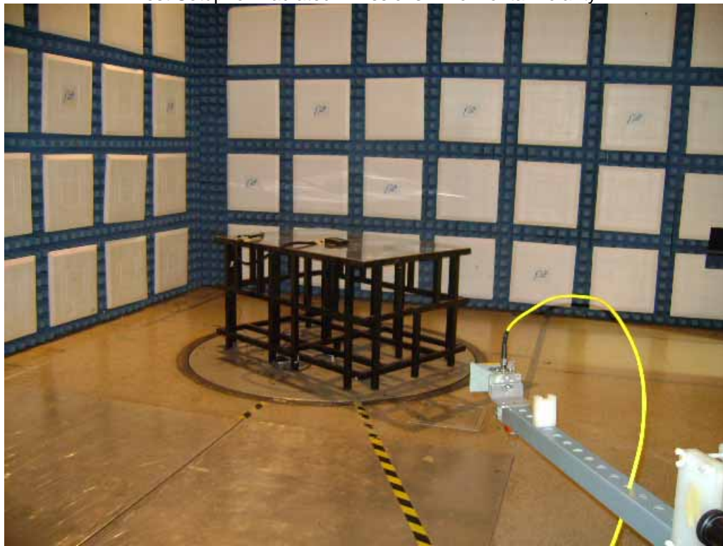
Test Setup for Radiated Emissions – Vertical Polarity
