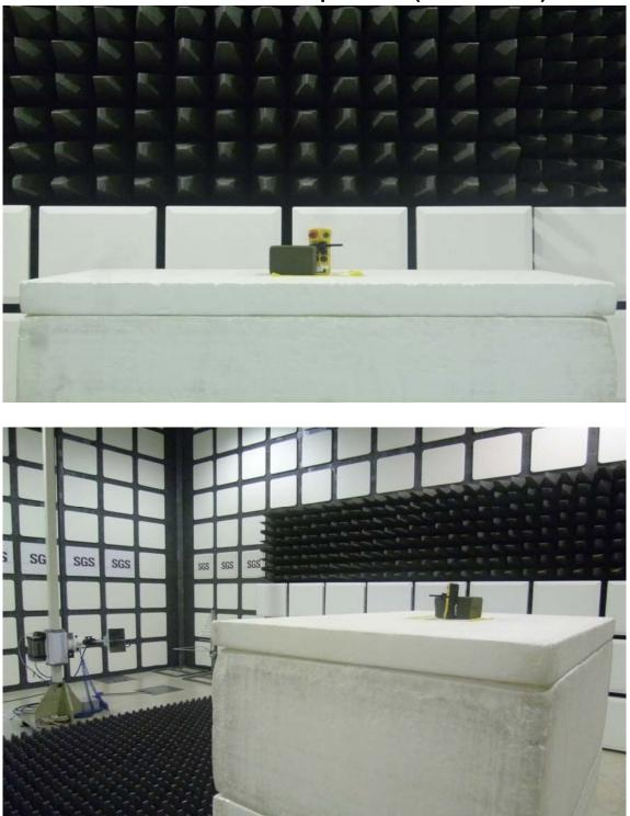
Radiated Emission Set up Photos (Above 1GHz)
