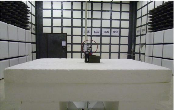
Radiated Emission Set up Photo (Below 1GHz)
