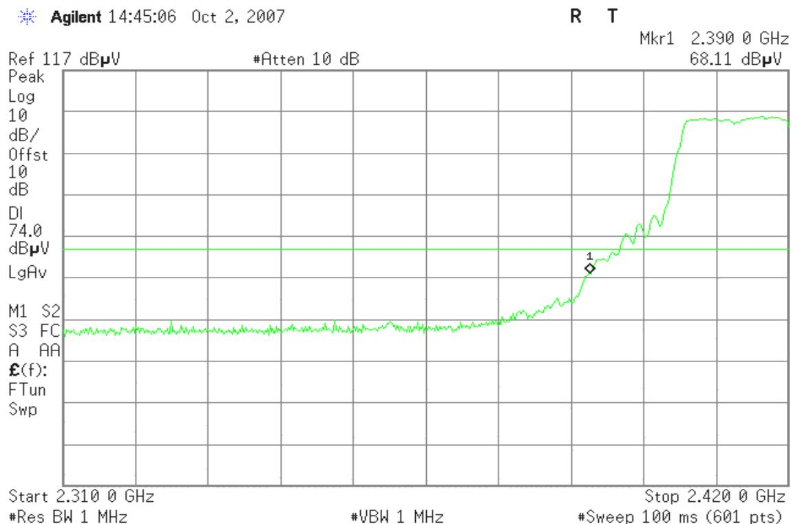
**Detector mode: Average****Polarity: Horizontal**
