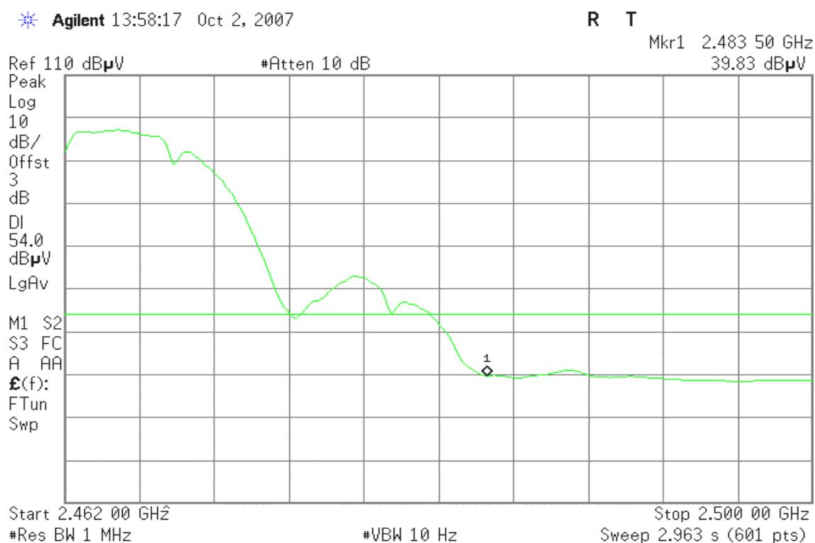
**Detector mode: Peak****Polarity: Horizontal**
