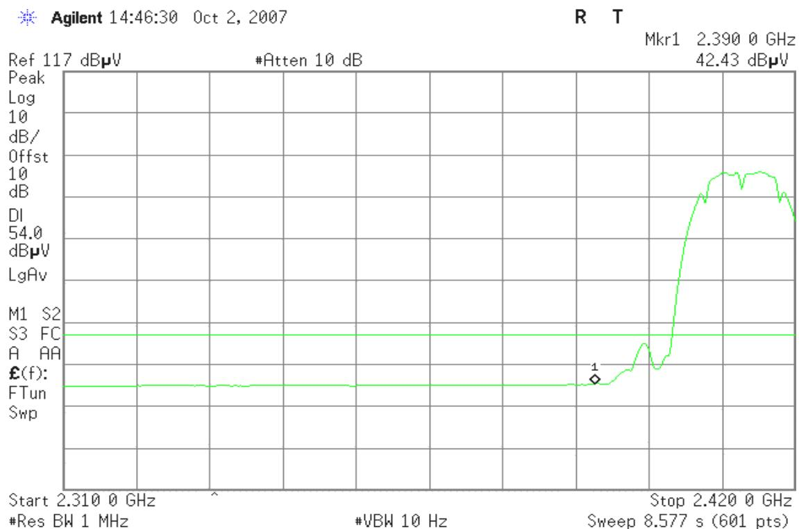
**Band Edges (IEEE 802.11b / CH High)****Detector mode: Peak****Polarity: Vertical**
