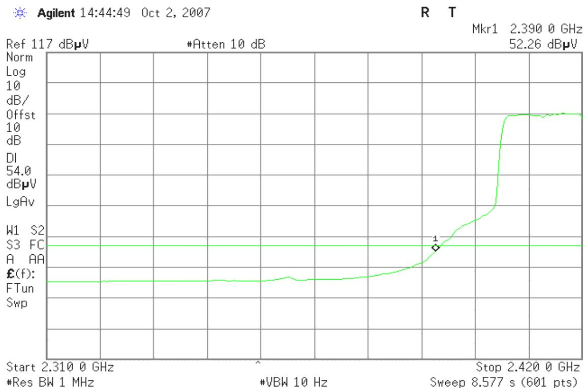
**Band Edges (IEEE 802.11g / CH High)****Detector mode: Peak****Polarity: Vertical**
