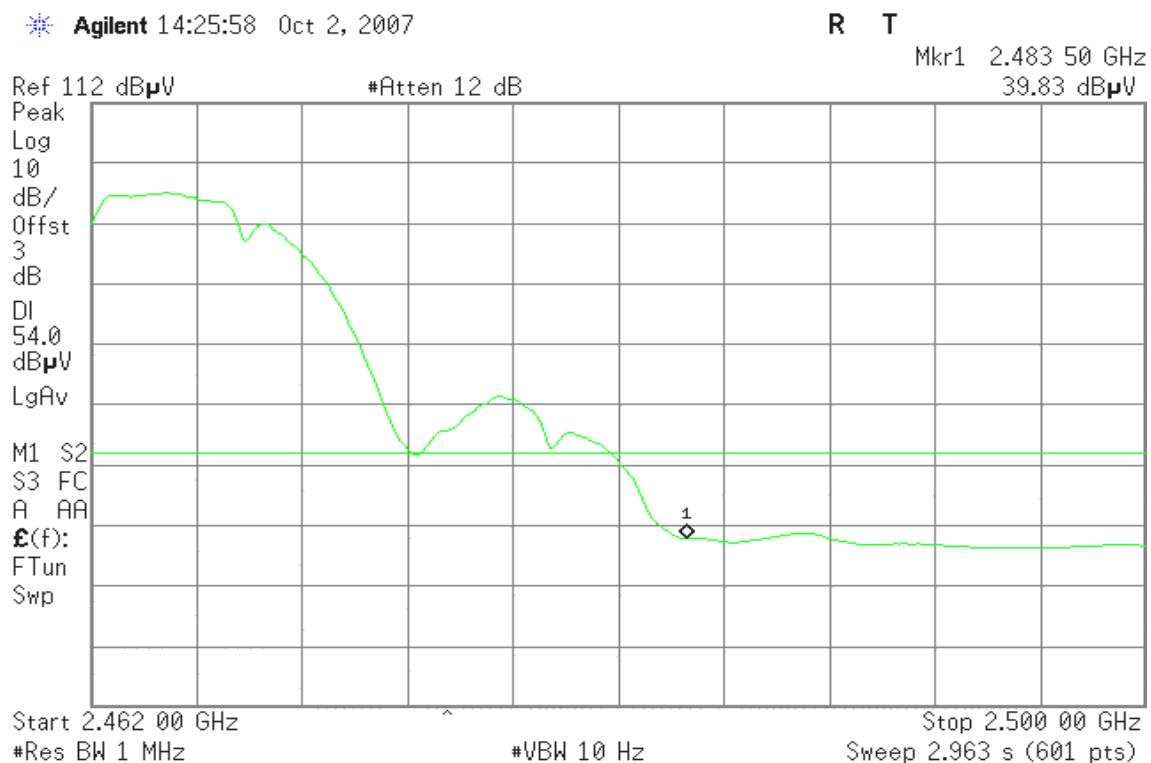
**Band Edges (IEEE 802.11g / CH Low)****Detector mode: Peak****Polarity: Vertical**
