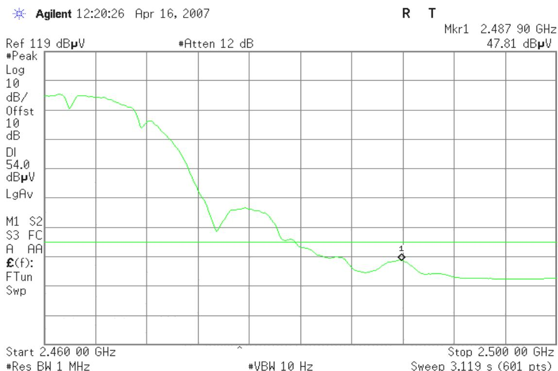
**Detector mode: Peak****Polarity: Horizontal**
