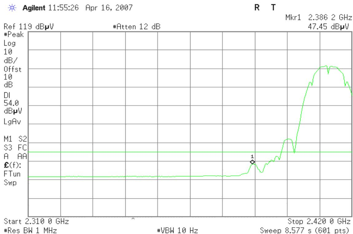
**Detector mode: Peak****Polarity: Horizontal**
