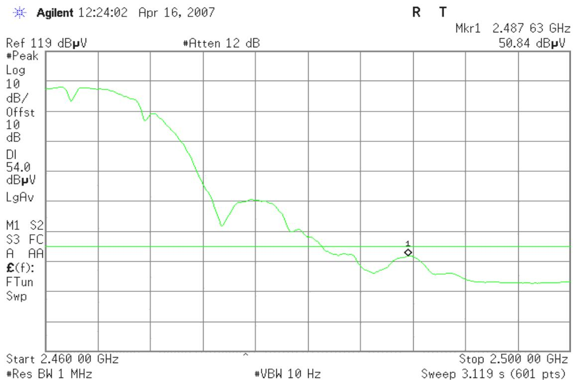
**Band Edges (IEEE 802.11g / CH Low)****Detector mode: Peak****Polarity: Vertical**
