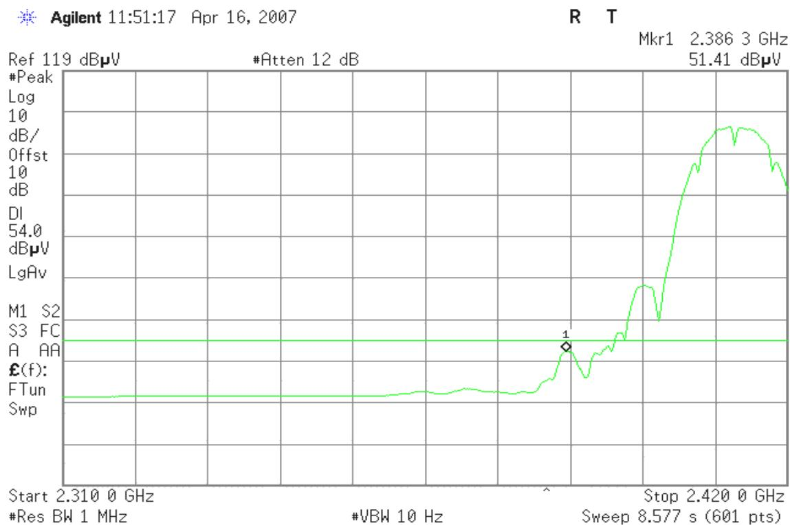
**Band Edges (IEEE 802.11b / CH High)****Detector mode: Peak****Polarity: Vertical**
