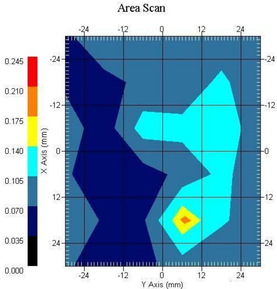
**802.11b, Main Antenna, EUT Back Z-Axis plot****Channel: 1**
