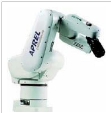
ALSAS-10U utilizes a six axis articulated robot, which is controlled using a Pentium based real-time movement controller. The movement kinematics engine utilizes proprietary (Thermo CRS) interpolation and extrapolation algorithms, which allow full freedom of movement for each of the six joints within the working envelope. Utilization of joint 6 allows for full probe rotation with a tolerance better than 0.05mm around the central axis.
