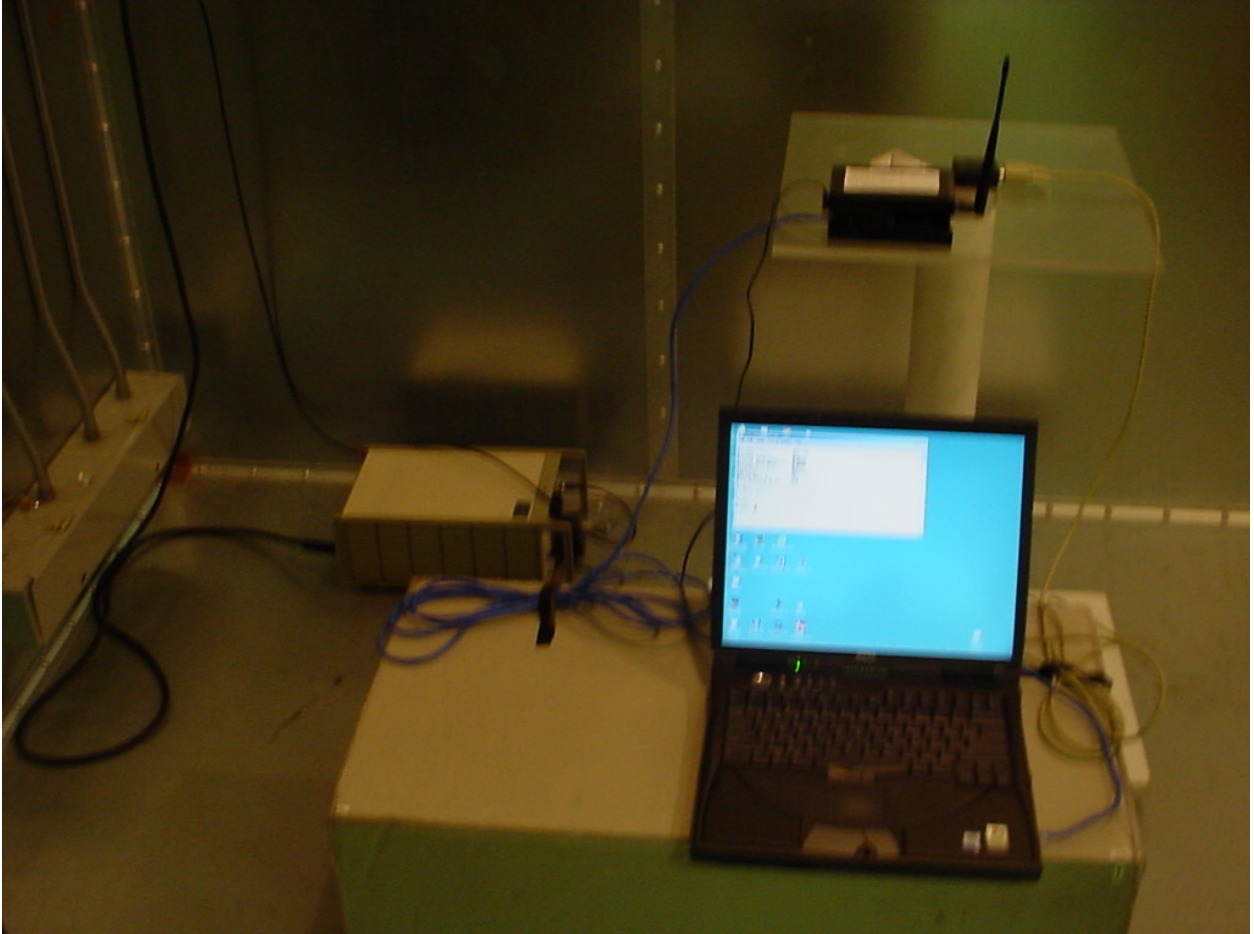
Setup for the Conducted Emissions Test
