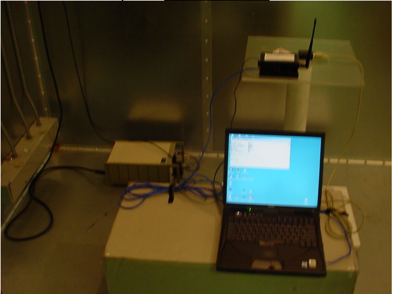
Setup for the Conducted Emissions Test
