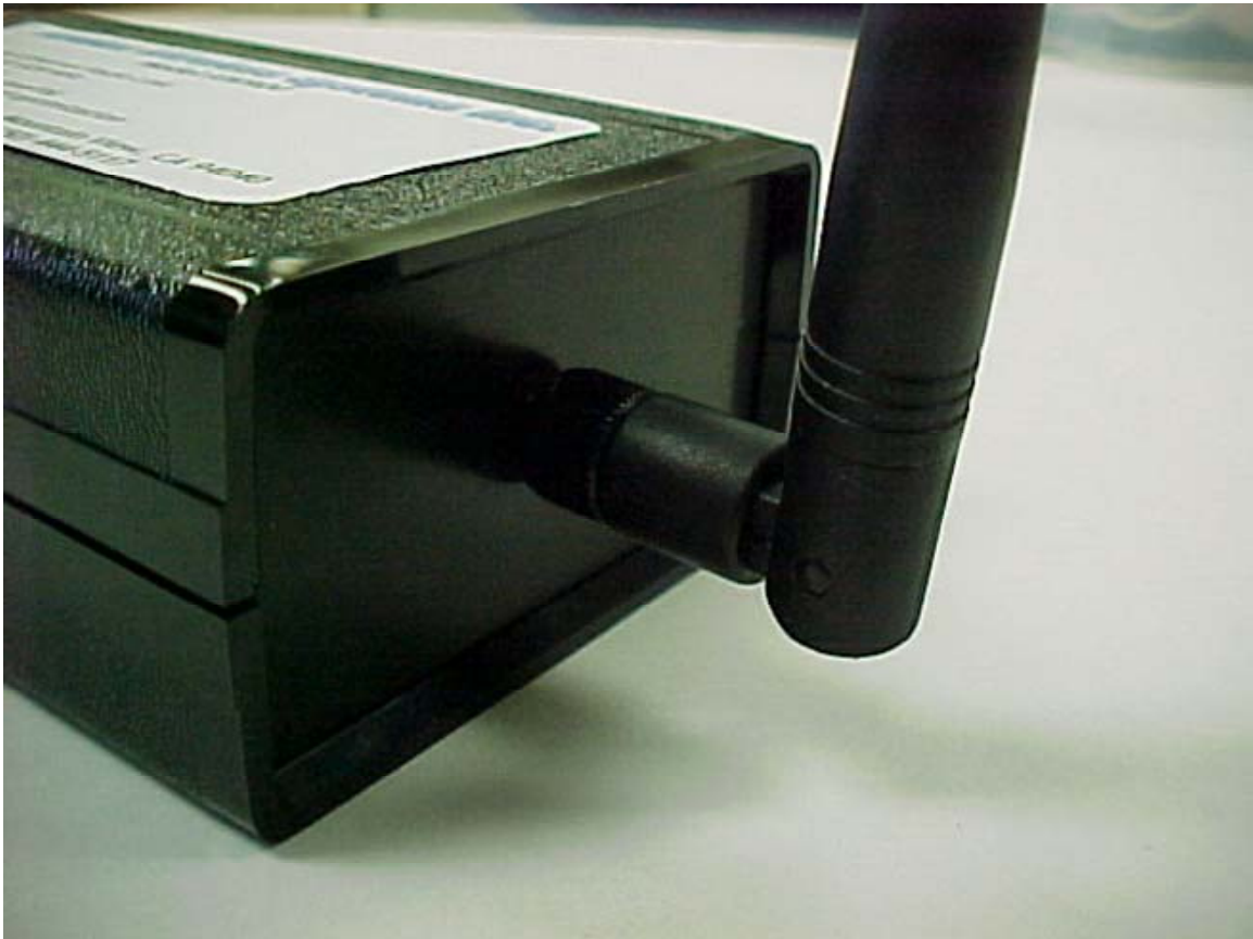
Photo Three – External Antenna Connection
