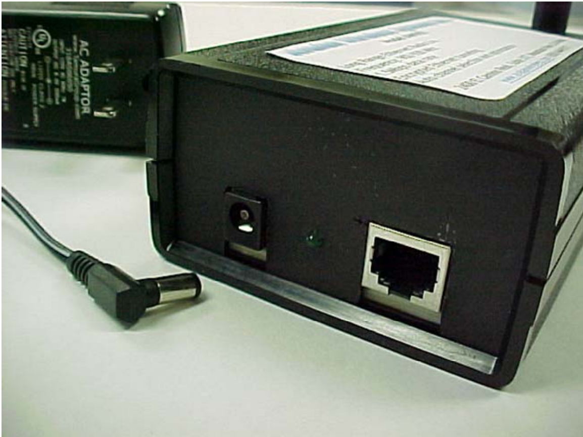
Photo Two – External Power Connection and Ethernet Port
