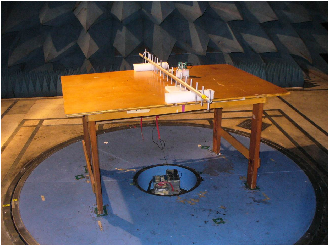
Figure 8: Radiated Emissions – EUT with Yagi Antenna (Front View)
