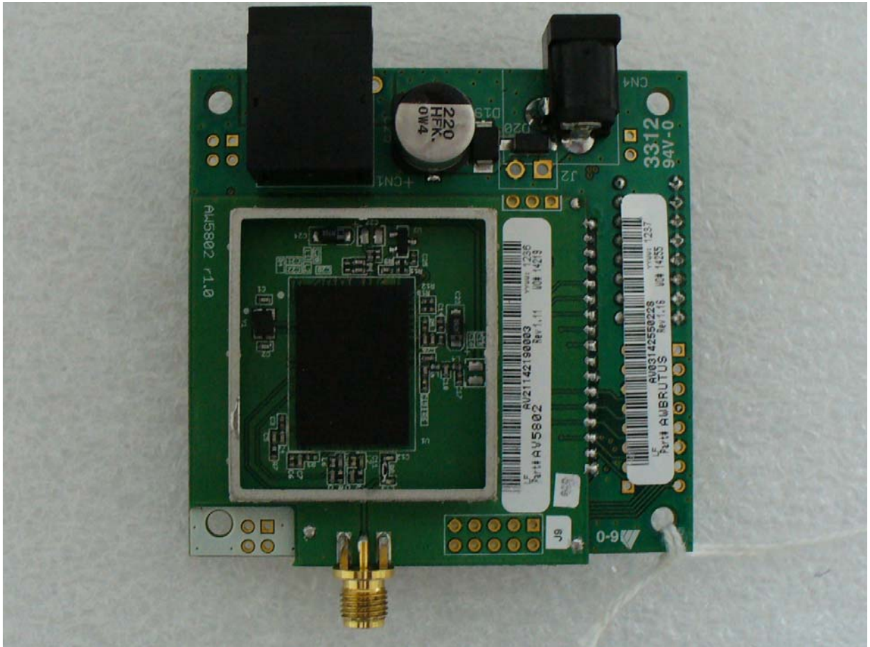
Figure 1: Top View (without shielding) – mounted on Ethernet board
