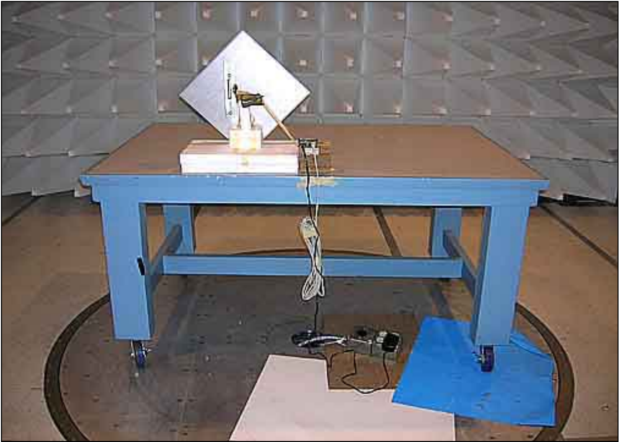
Radiated Emissions - Back View Receiver Panel Antenna 15.109
