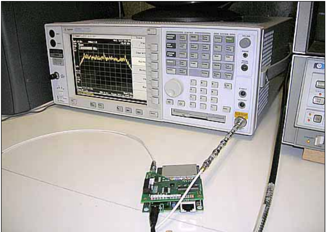
RF Power (15.247(b)(3)) and Peak Power Spectral Density (15.247(e))
