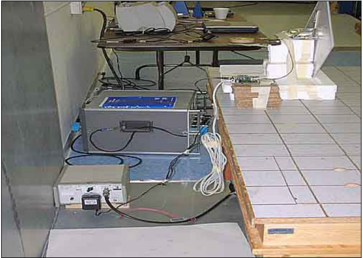
Mains Conducted Emissions - Side View 15.107 & 15.207
