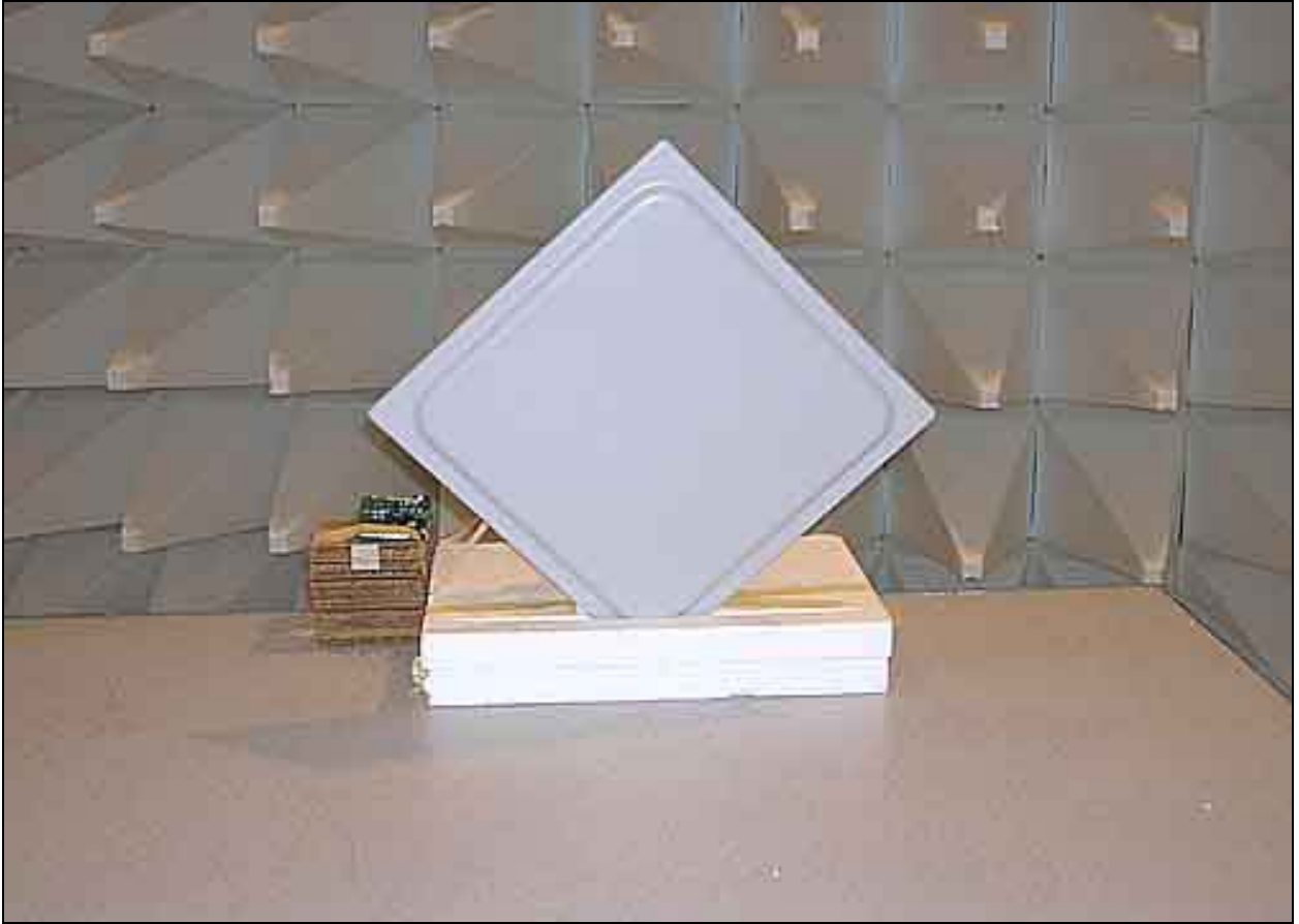
Radiated Emissions - Front View Receiver Panel Antenna 15.109
