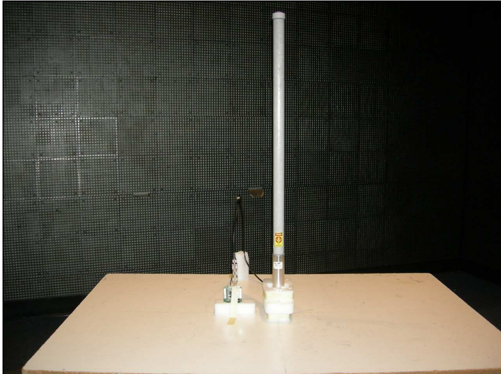
Figure 3: Radiated Emissions – Y Position Omni-Directional (Center fed Collinear Dipole Array) Antenna
