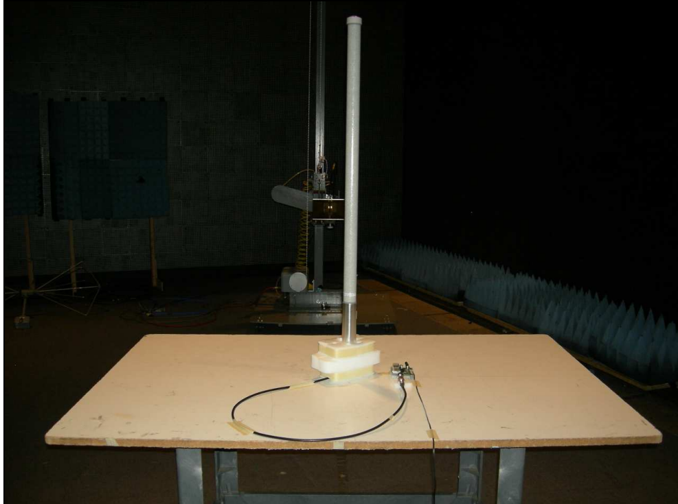
Figure 2: Radiated Emissions – X Position (Rear View) Omni-Directional (Center fed Collinear Dipole Array) Antenna
