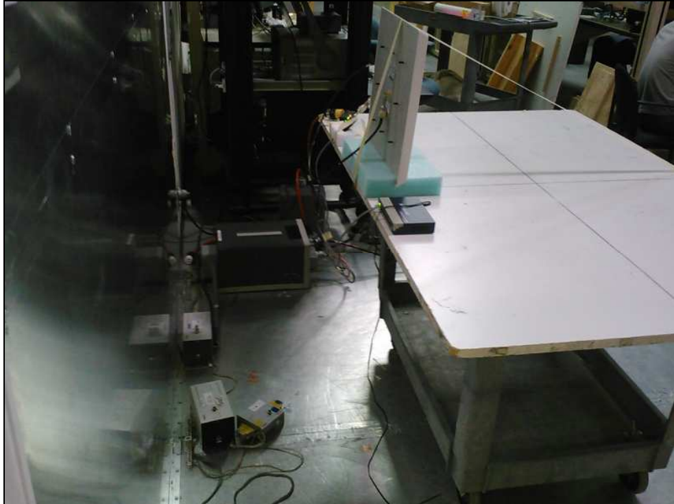
Figure 18: Conducted Emissions – Side View Panel Antenna
