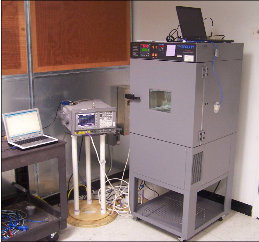
Photograph 5. Frequency Stability, Test Setup
