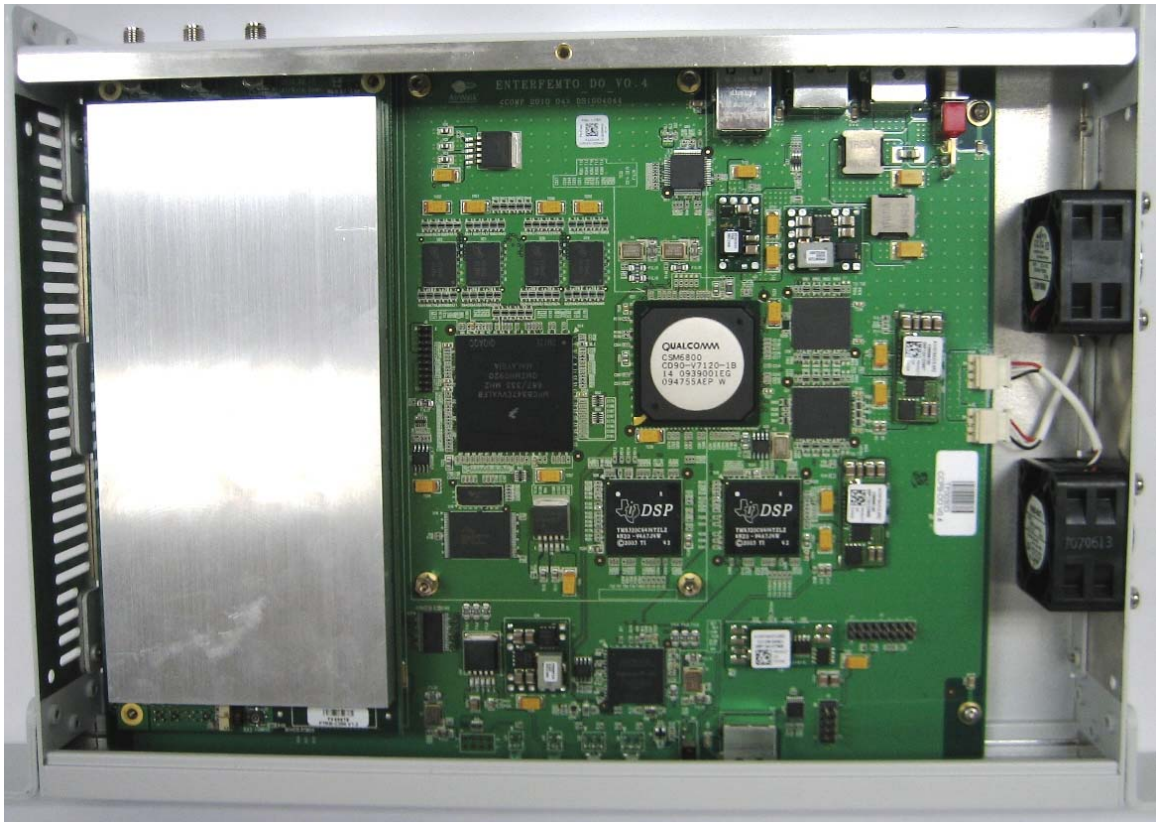
Photograph 2. Digital Board with FTRB
