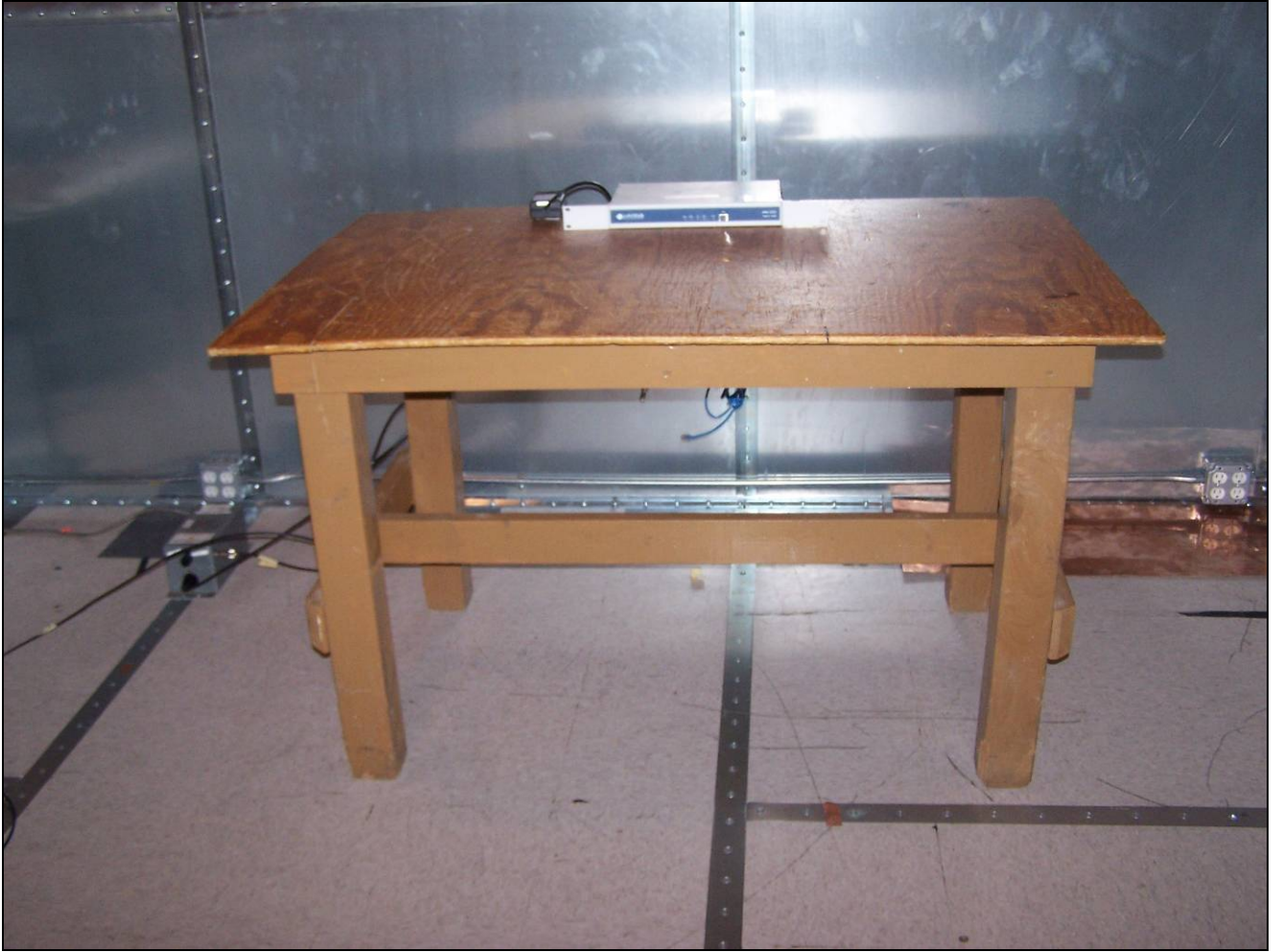
Photograph 1. Conducted Emissions, Test Setup
