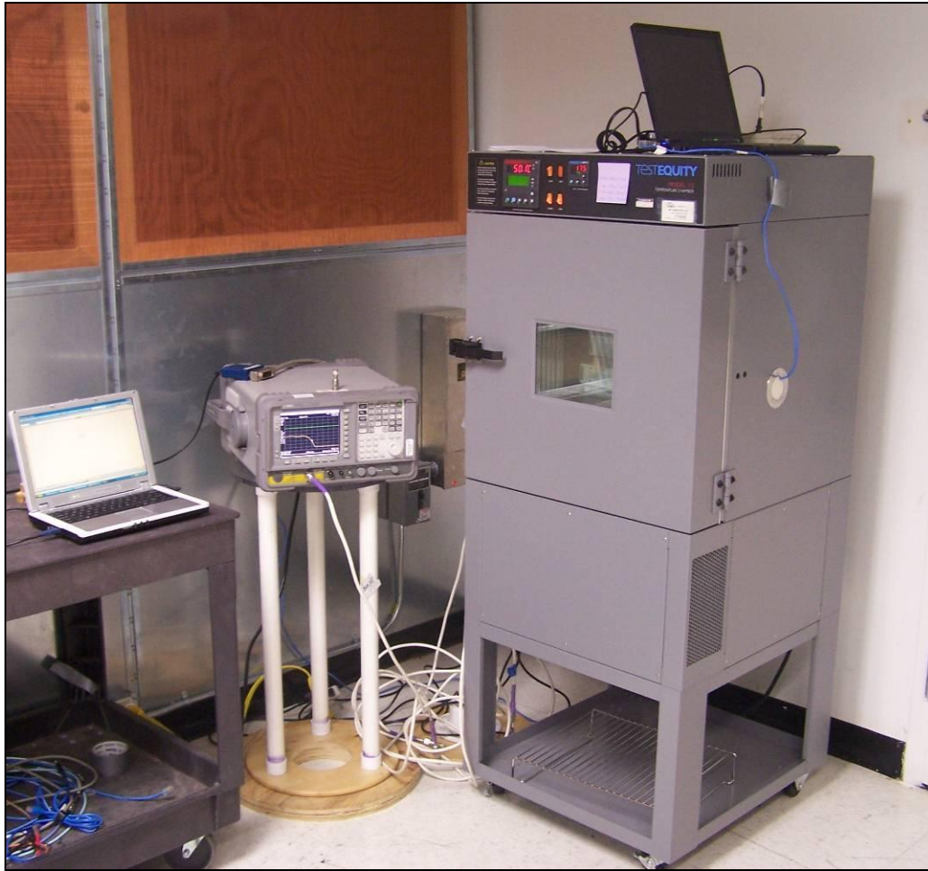
Photograph 5. Frequency Stability, Test Setup
