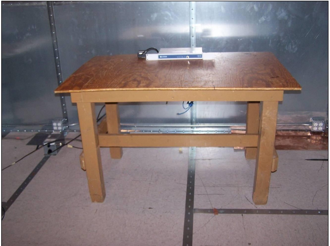
Photograph 1. Conducted Emissions, Test Setup
