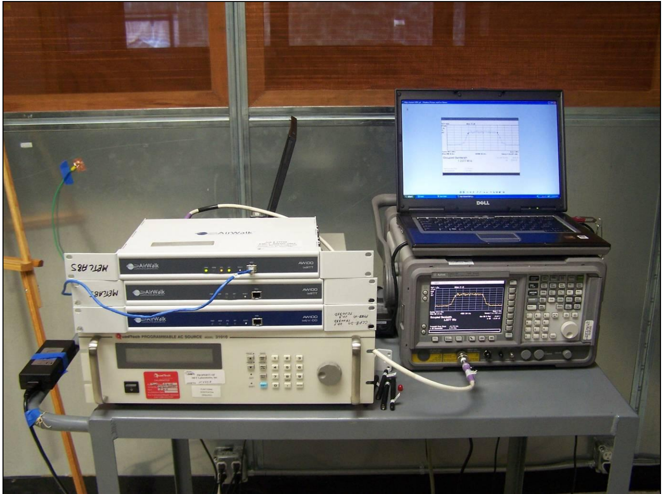
Photograph 3. Occupied Bandwidth, Test Setup
