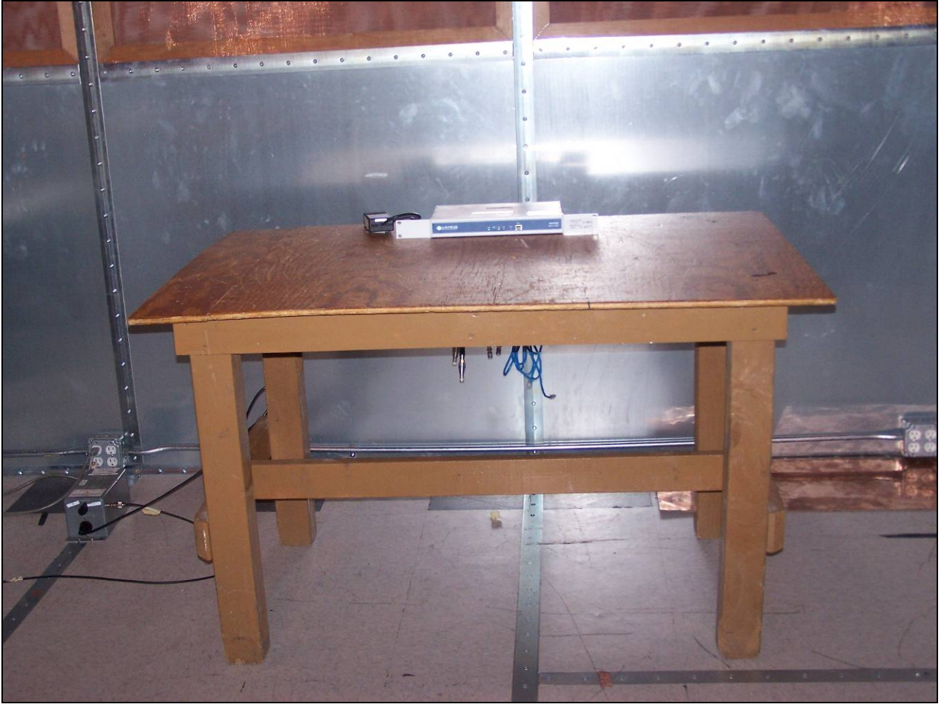
Photograph 1. Conducted Emissions, Test Setup
