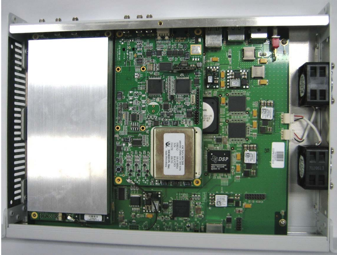
Photograph 1. AW100 800MHz 200mW - Digital Board with FTRB and GTIB
