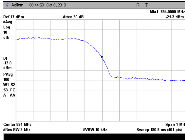
Plot 50. Frequency Stability, High Channel, 10°C
