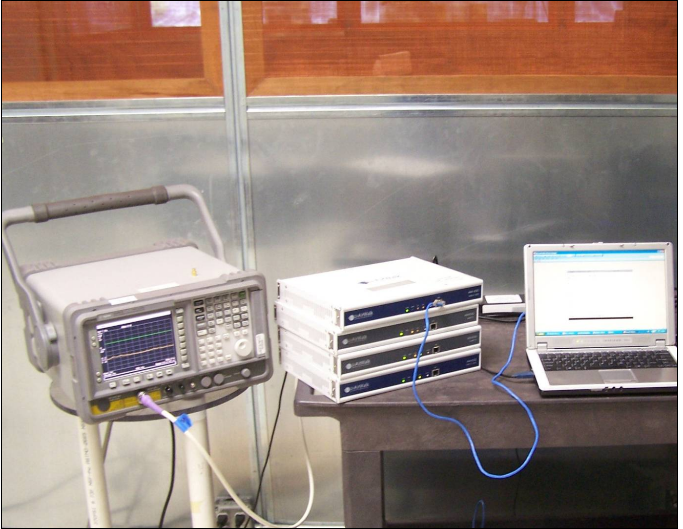
Photograph 3. RF Power Output, Test Setup
