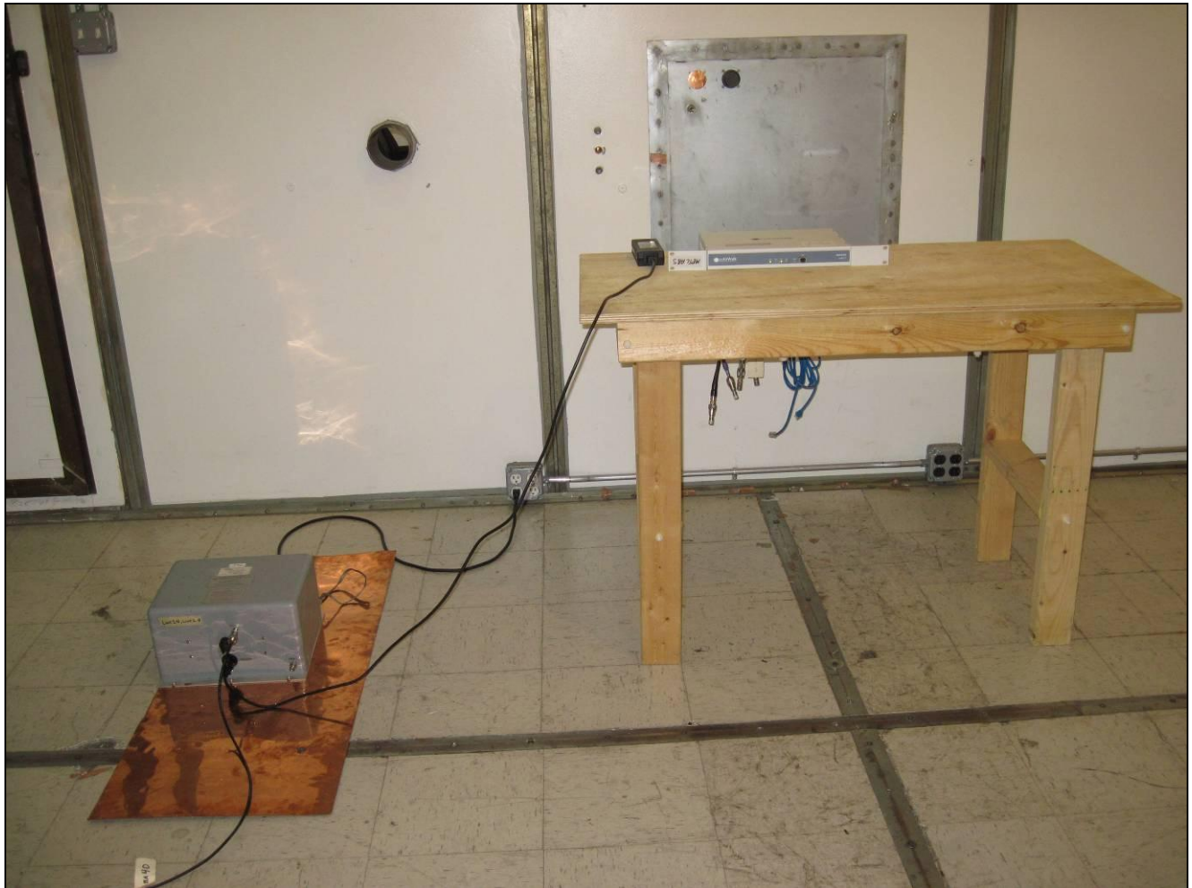
Photograph 1. Conducted Emissions, Test Setup
