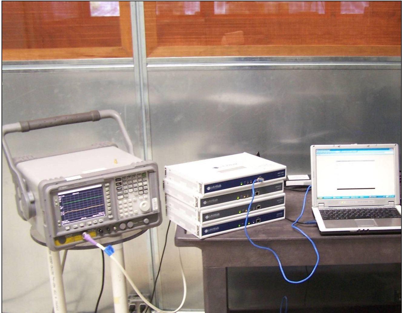
Photograph 3. RF Power Output, Test Setup
