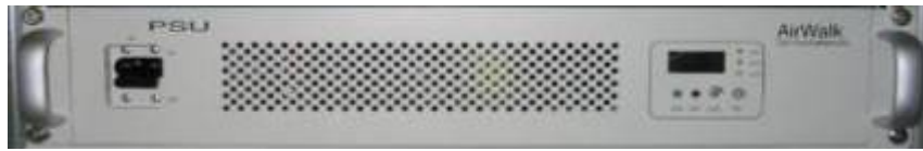
Figure 5-12 Sector RU PSU - Photo (Front View)
