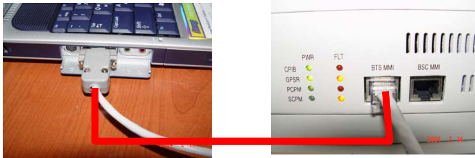
Figure 7-2 - PC to AW 96 Cable Connection Diagram
