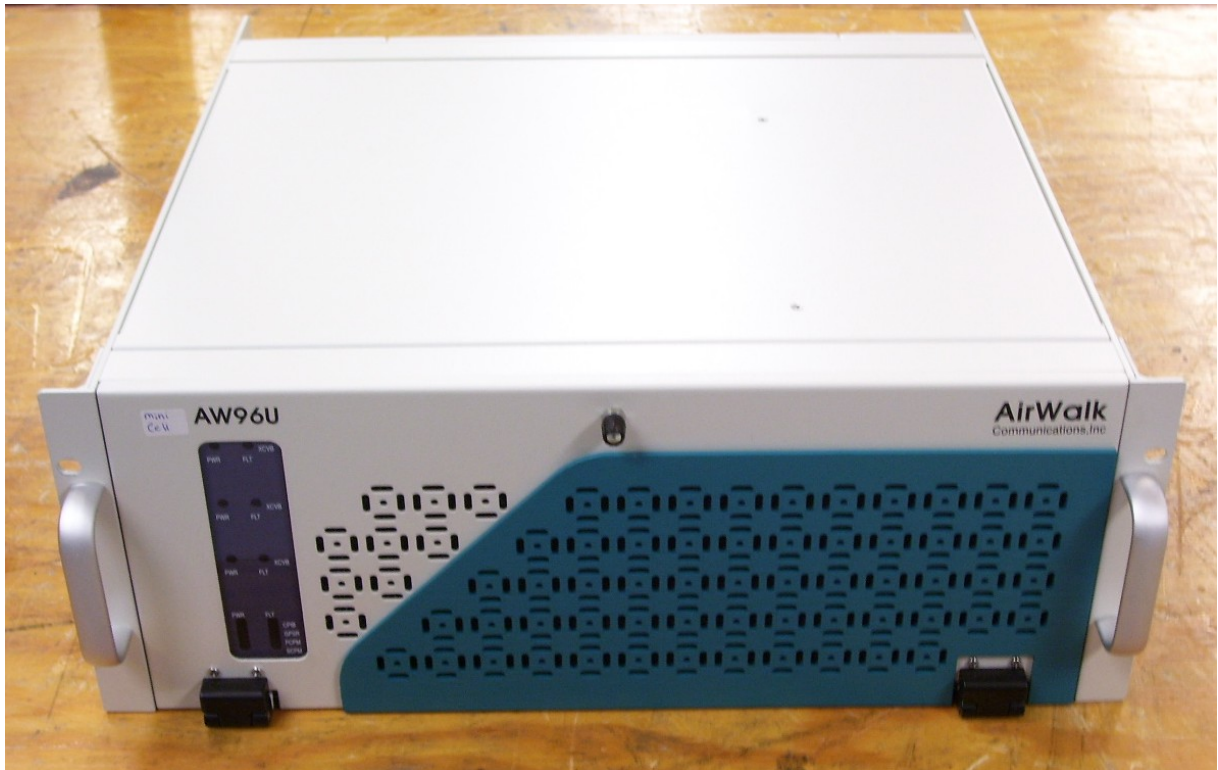
Photograph 1. AW-96 Pilot Beacon
