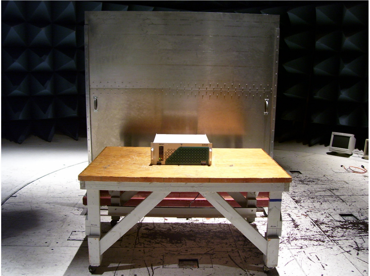
Photograph 2. Conducted Emissions Test Setup
