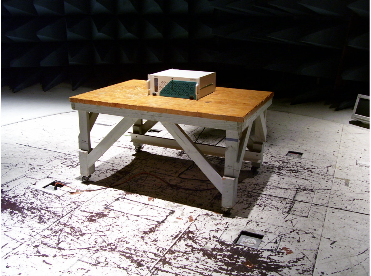
Photograph 3. Radiated Emission Limits Test Setup
