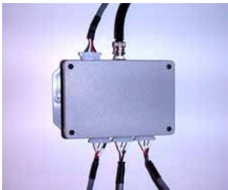
Figure 10 - Matching Board cable connected to Match Board Box.
