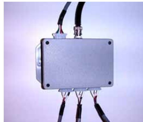
Figure 13 - Antenna Cable to Matching Board Box Connection
