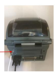
1) Attach the antenna cable at this this location in the back of the printer.
