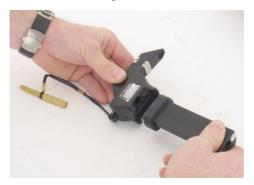
2. Attach the SAAD to the front end of the RPG-7.
