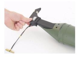
3. Rotate the optics of the SAAD into the line of sight. A reticle pattern will be visible.
