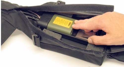
1a. Install the 1-cell battery in the body harness.
