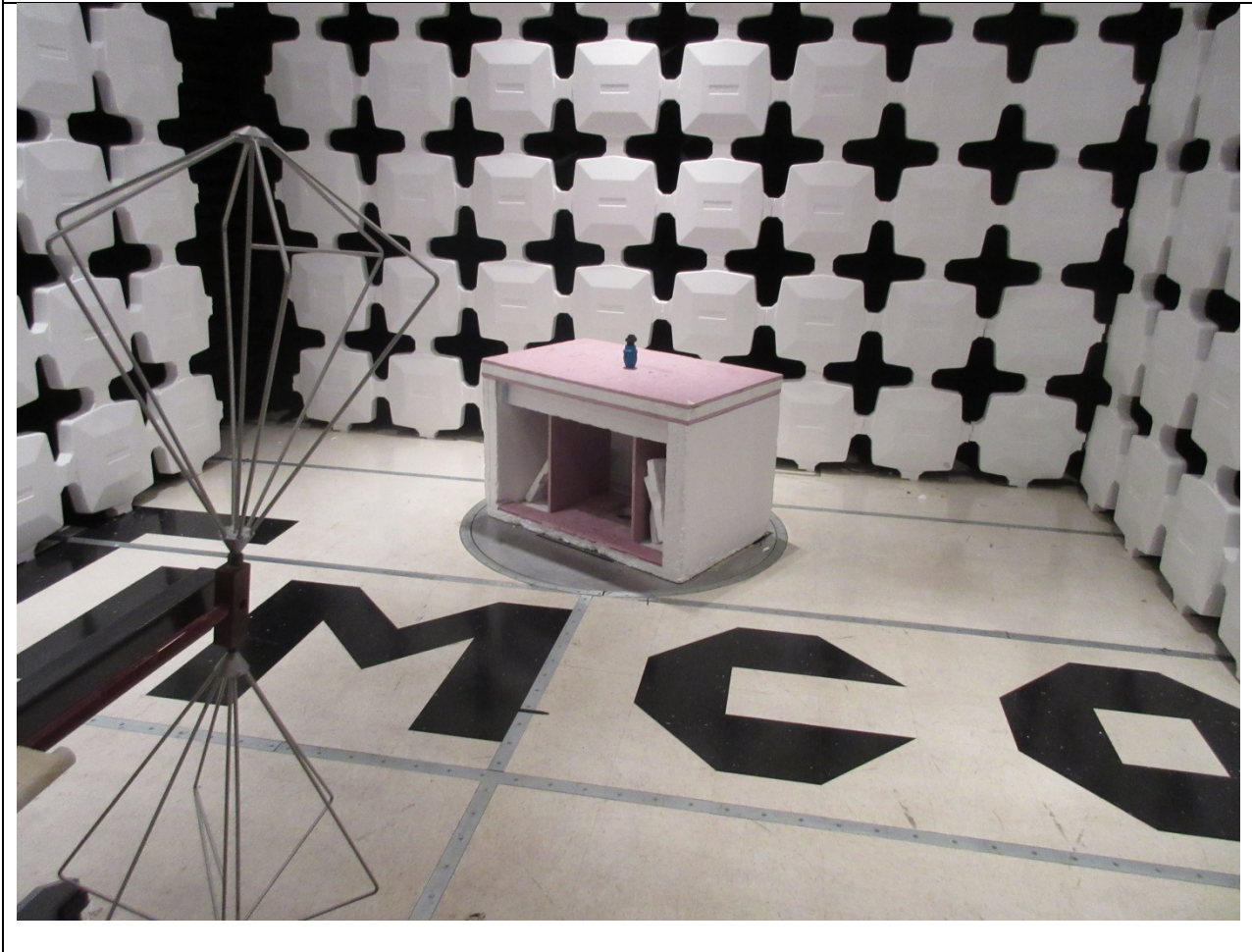
Radiated Emissions Below 1 GHz Setup
