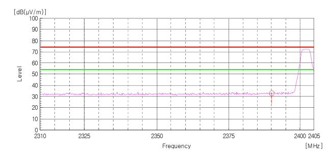
AV Detector: RBW: 1 MHz, VBW: 10 Hz (2 310 MHz - 2 405 MHz), Worst case (Low, Horizontal)
