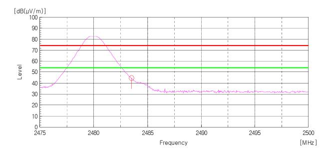
AV Detector: RBW: 1MHz, VBW: 10 Hz (2 475.0 MHz - 2 500.0 MHz), Worst case (High, Horizontal)
