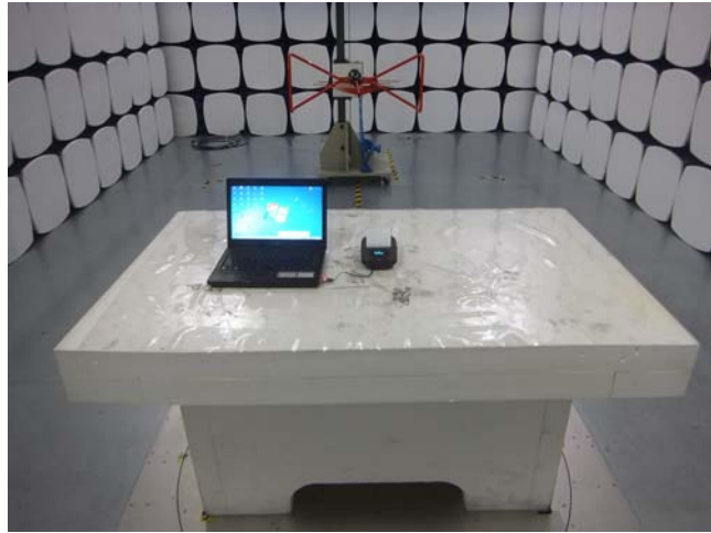
Radiated Spurious Emissions Test Setup Below 1GHz
