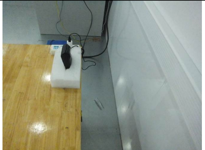
Conducted Emissions Test Setup Side View
