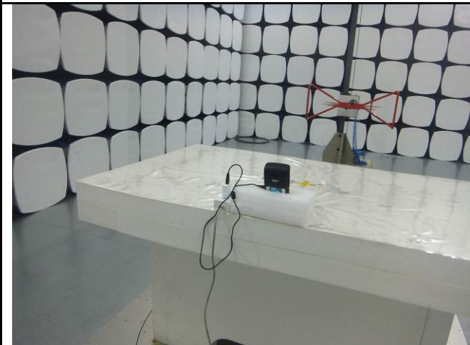
Conducted Emissions Test Setup Front View
