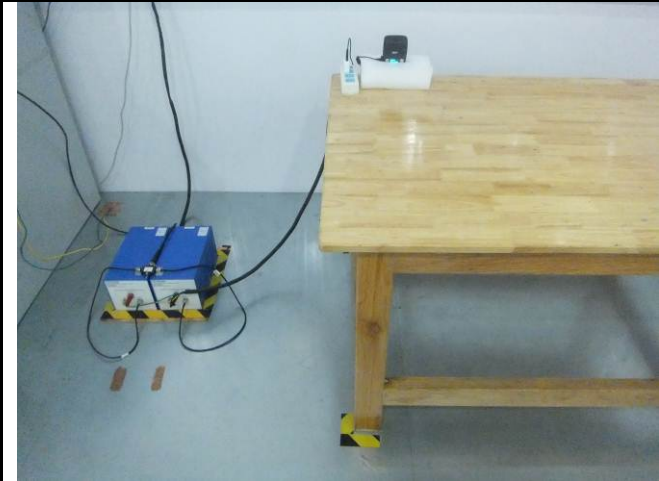
Conducted Emissions Test Setup Front View
