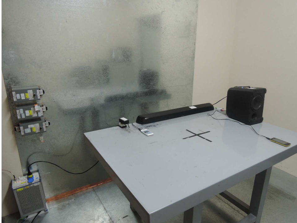
Photograph 6: Set-up for for Mains Conducted testing Front
