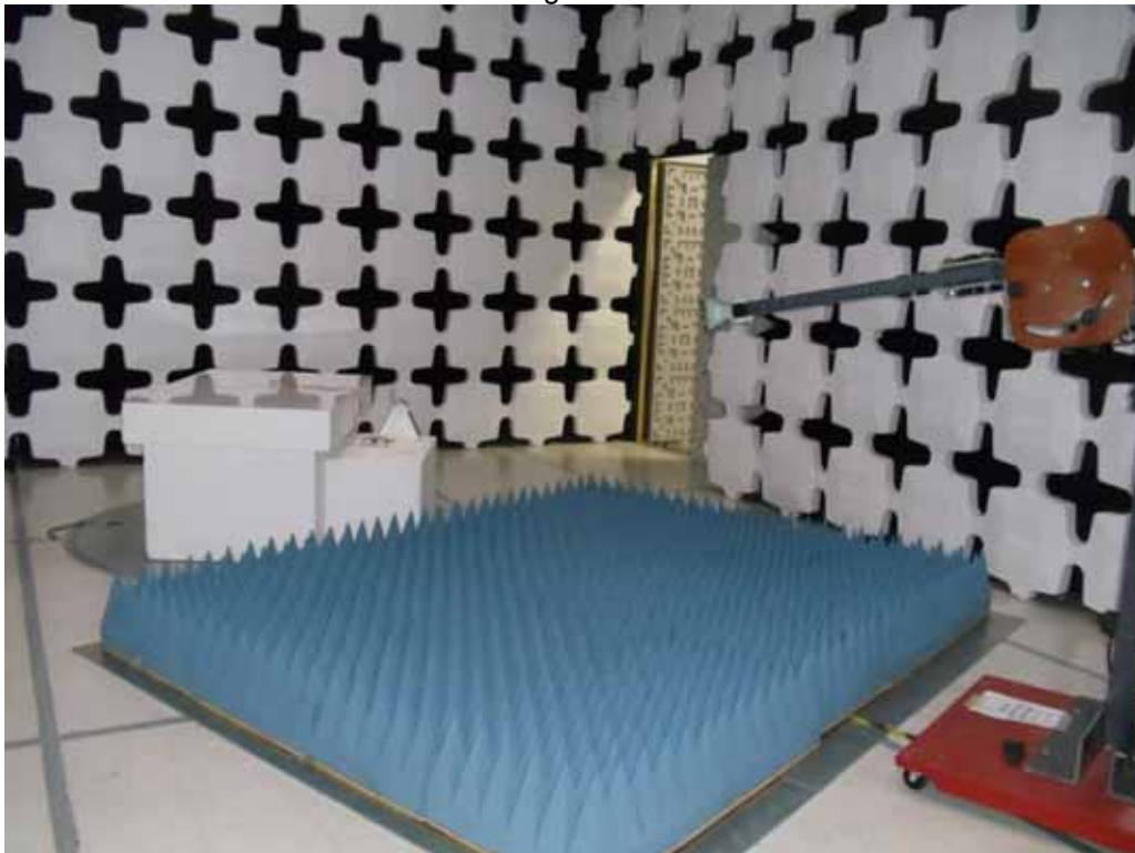
Test Setup for Radiated Emissions, Above 1GHz – Horizontal Polarization
