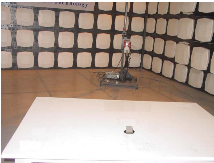
Figure 2 Test photo of Transmitter Spurious Emission (TX Mode above 1G)
