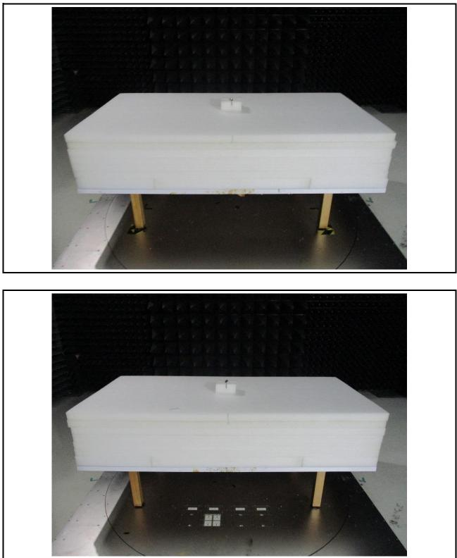
Radiated Emission Below 30MHz Test (Battery mode)
