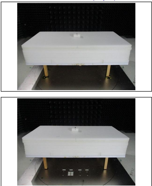
Radiated Emission Below 1 GHz Test (Battery mode)
