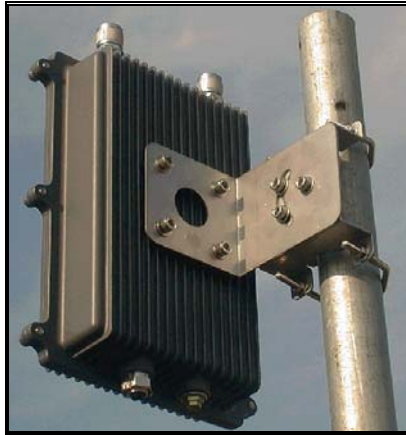
Figure 2-17 Install Outdoor Unit to the Mast
