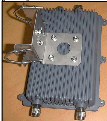
Figure 2-16 Attach the Mounting Bracket to Outdoor Unit
