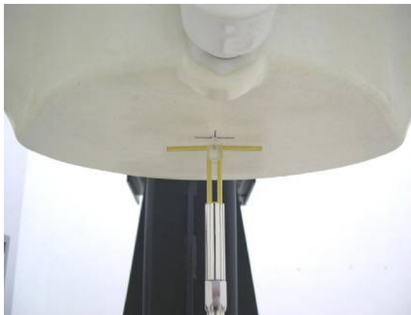
Picture 8.2 Photo of Dipole Setup
