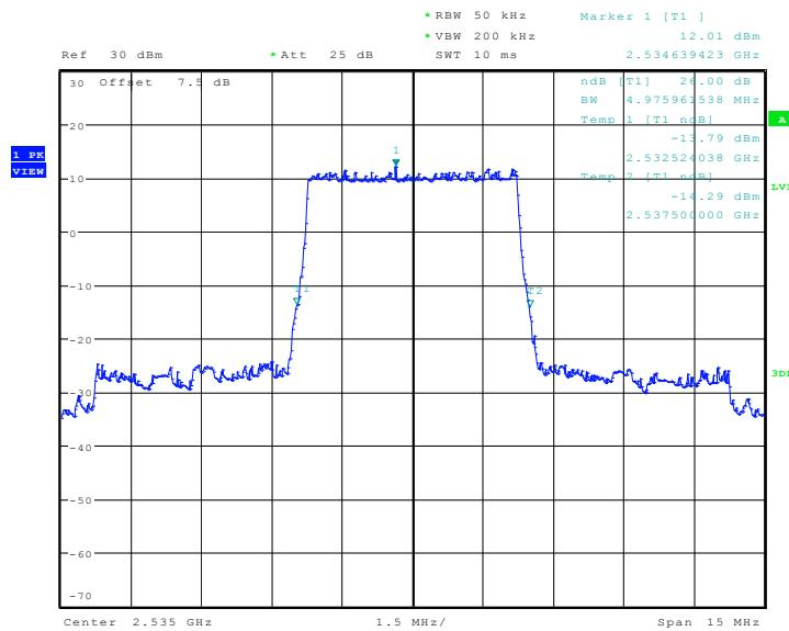
**LTE band 7, 5MHz Bandwidth,16QAM (-26dBc BW)**
