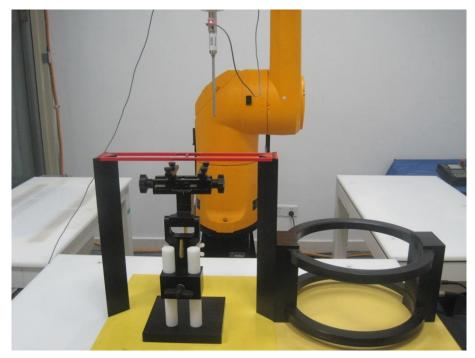
Picture A1: HAC T-Coil System Layout
