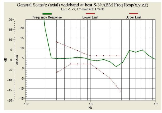
Figure C.2 Frequency Response of GSM 1900
