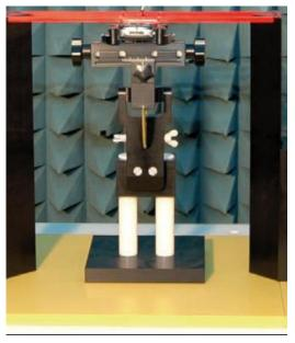
Figure 6.4 HAC Phantom & Device Holder
