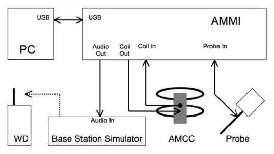
Figure 6.2 T-Coil setup with HAC Test Arch and AMCC
