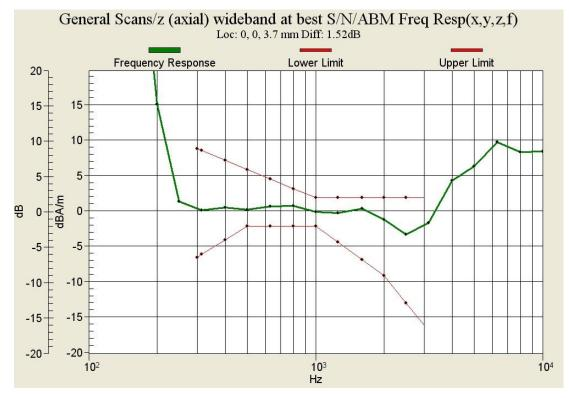
Figure C.1 Frequency Response of GSM 850
